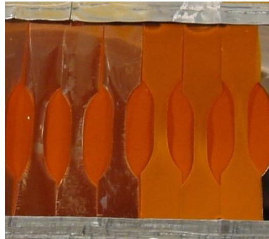
Figure 3. 8% PTFE-SiO x /CP1 (three samples on the left) showing evidence of cracking of the surface coating and uncoated Kapton E (3 samples on the right) showing matte surface post flight.
