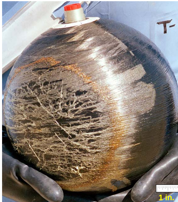
Figure A-7 Level II Discoloration (Chemical Exposure)
