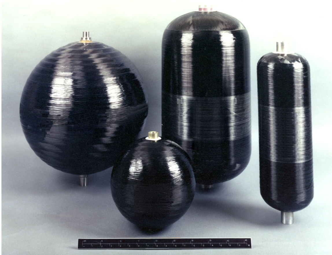
Figure 1 Flight-qualified COPVs Used to Test and Evaluate Visual Inspection Indications and Reductions in Strength
