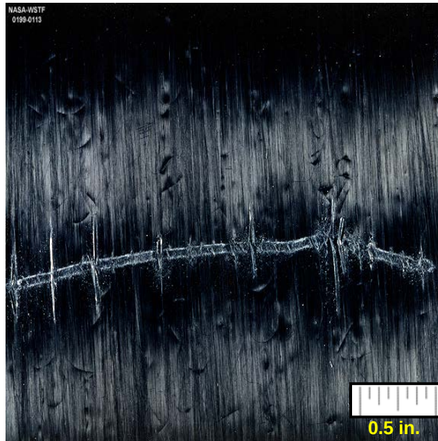
Figure A-5 Level II Scratch/Scuff/Abrasion (Cut Tows)
