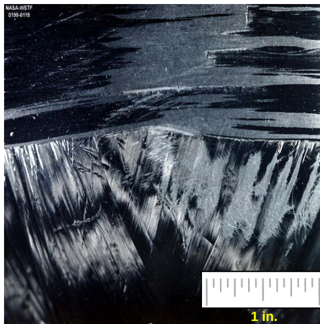
Figure A-4 Level I Scratch/Scuff/Abrasion (Matrix Grinding)
