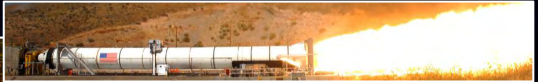
5-Segment Solid Rocket Booster development motor test, Promontory, UT, Sep 2011.
