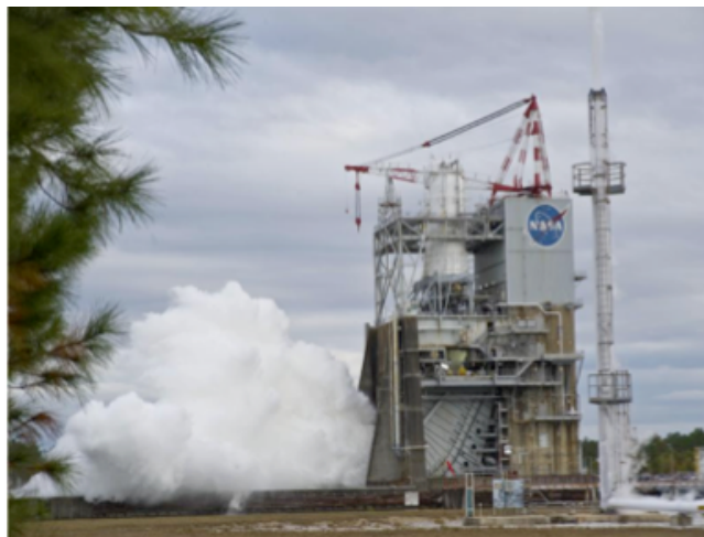
J-2X 500-sec test firing at SSC
