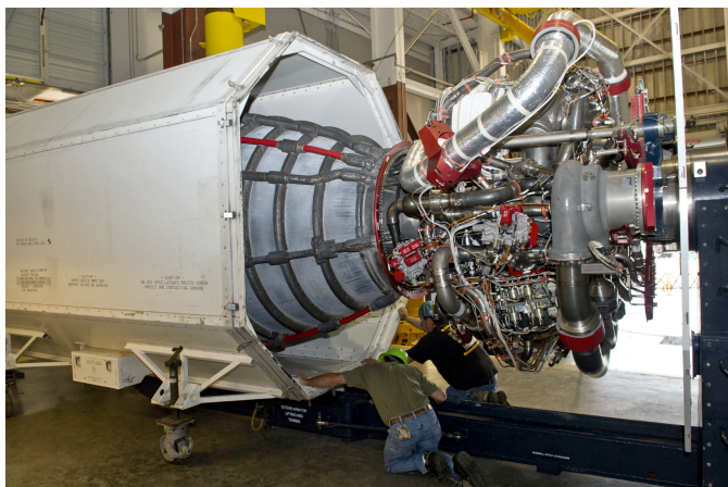
Figure 4. SLS RS-25 core stage engine being transported for storage and green-run testing.
