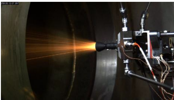
Fig. 7: Thruster testing at WSTF
