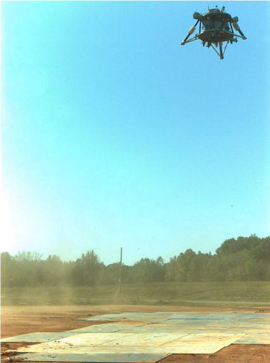
Fig. 7: WGTA outdoor test flight, altitude 10 meters
