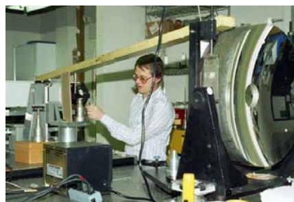
Figure 7: Hindle Sphere test setup to measure the Spitzer Telescope secondary mirror. A 2x4 is used to structurally connect the interferometer phase modulation head and Hindle sphere to minimize vibration induced relative motion. (Photo Courtesy of Goodrich Corporation)
