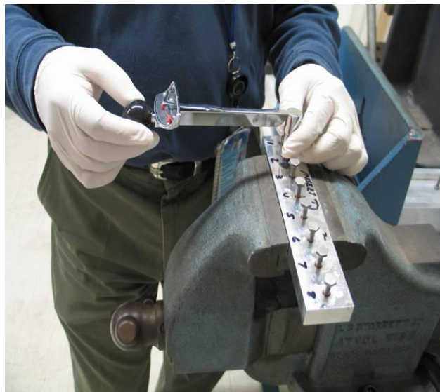
FIGURE 5 - BREAKAWAY TORQUE MEASUREMENT IN OFF DIRECTION
