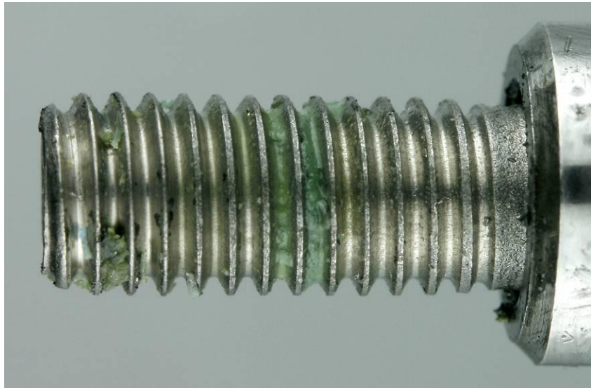
FIGURE 30 - AFTER VIBRATION TEST - LOCTITE APPLIED TO NUT ELEMENT ONLY
