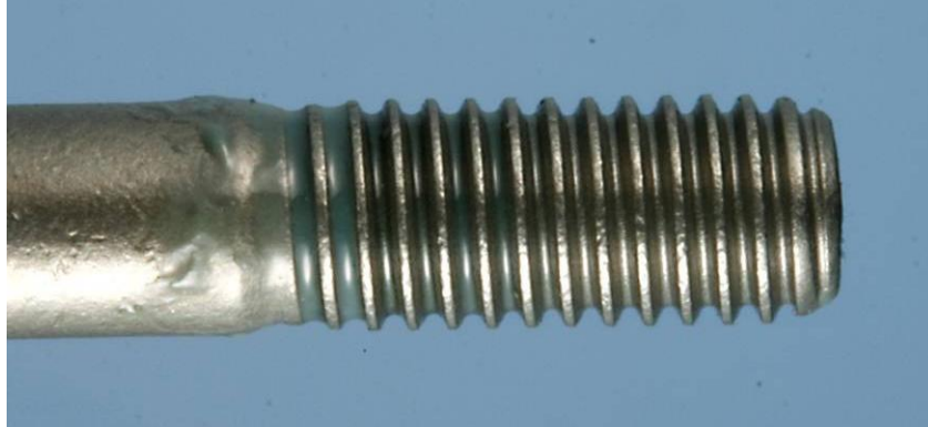
FIGURE 18 - LOCTITE 242 REMOVED FROM HENKEL TEST
