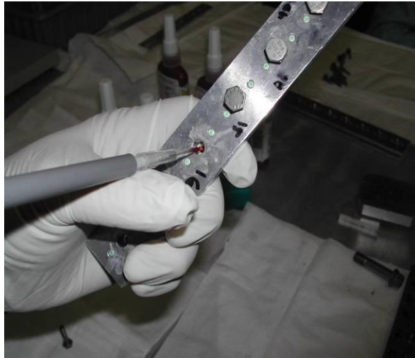
FIGURE 7 - LOCTITE APPLIED TO INTERNAL THREADS
