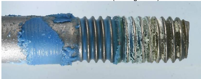
FIGURE 17 - LOCTITE 242 WITH 125% COVERAGE
