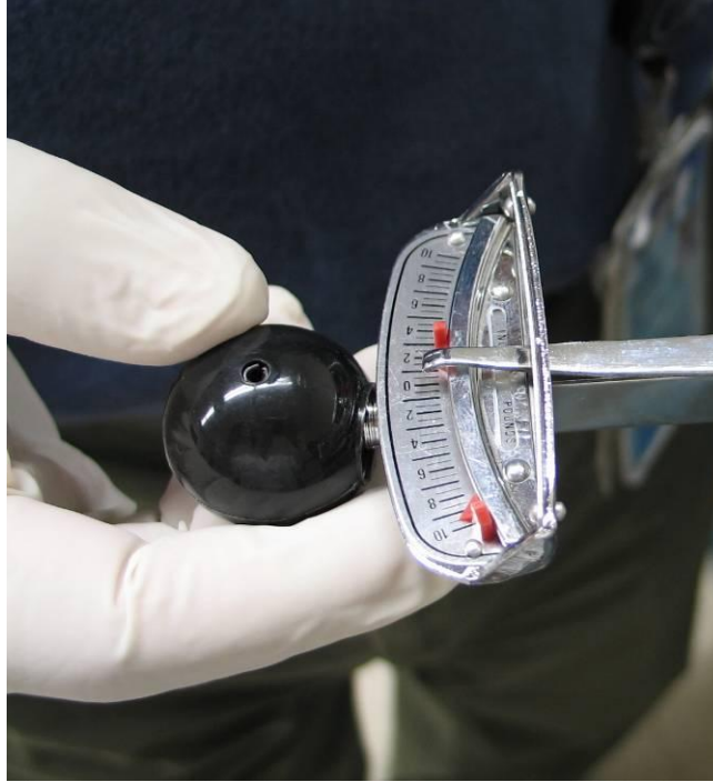
FIGURE 6 - MINIATURE TORQUE WRENCH, FULL SCALE = 10 INCH-POUNDS
