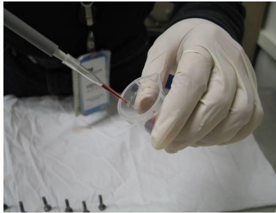
FIGURE 3 - LOCTITE DISPENSED FROM TARE CUP
