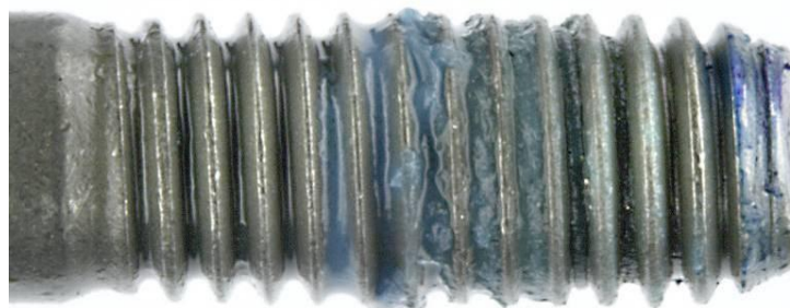
FIGURE 23 - LOCTITE APPEARANCE AFTER REMOVAL FROM NUTPLATE
