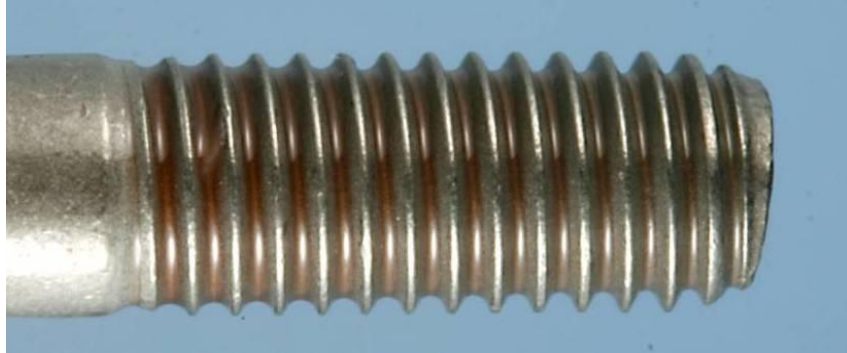
FIGURE 14 - BOLT WITH LOCTITE 078 REMOVED FROM HENKEL TEST
