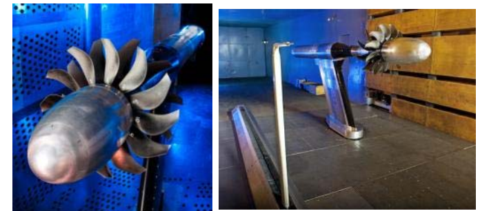
Open Rotor Propulsion Rig installed in GRC's 8x6 (left) and 9x15 (right) Wind Tunnels
