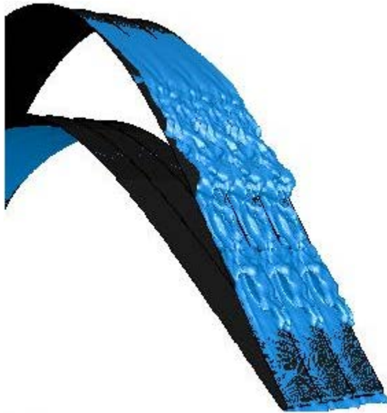
Figure 4.51: Isosurface of mean V_x = 0.01 m/s for Case (6), Re=50,000 , f=24 Hz, (F=0.56) , DC=10\%
