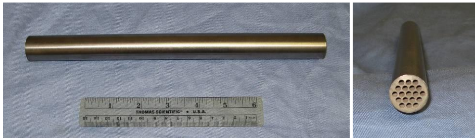
Figure 5. Images of a hexagonal fuel element sample during HIP fabrication.
