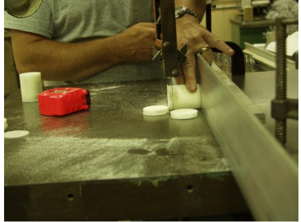
Figure 4. Specimen length manufacturing
