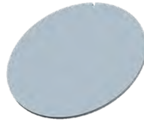
Figure 2. SSBD design showing the notch at the top disk in line with the grain direction of the shim stock.
