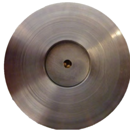
Figure 5. Petal catcher (middle) inserted toward the breach into the modified AR section showing the center of the etched SSBD underneath.
