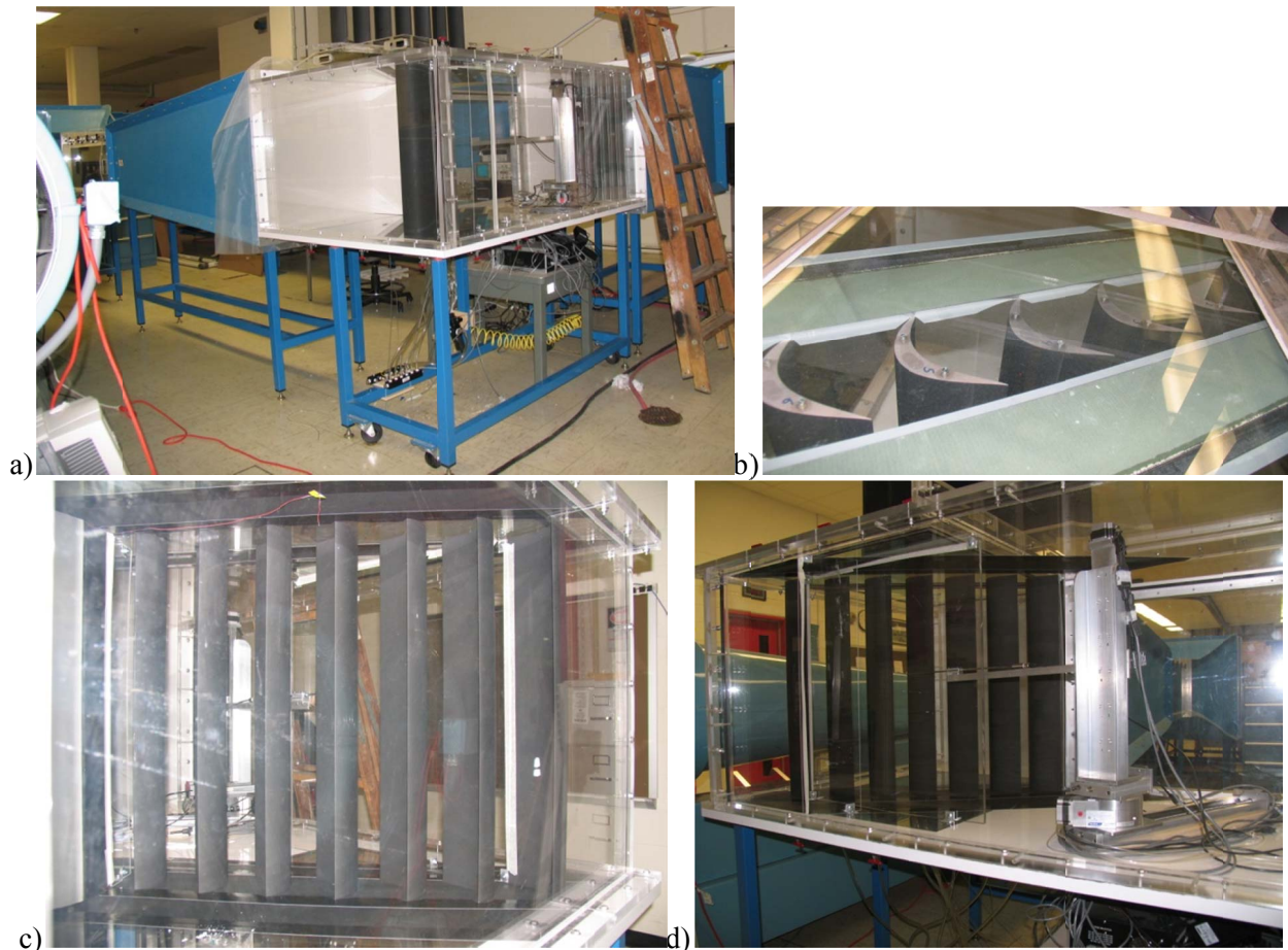
Fig. 1.2: Corner cascade test section, a) test section with fine screen visible at exit of diffuser and hardware below test section for producing pulsed VGJs, b) top view of cascade blades, c) view of cascade from upstream, d) view of cascade from downstream with traverse for probe movement to the right.
