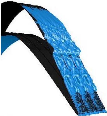
Figure 13. Isosurface of mean V_x = 0.01 m/s for Case (6), Re=50,000 , B=0.5 , F=0.56 , DC=10\% .
