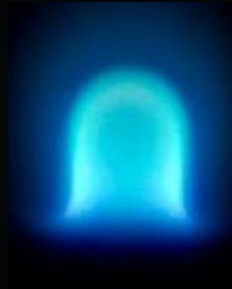
Image of a lifted flame of 50% propylene in a coflow of air (at ambient pressure) from an exploratory test conducted on the International Space Station in 2009 as part of the Smoke Point In Coflow Experiment (SPICE).
