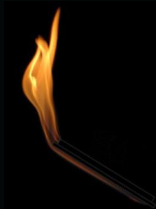
Image of a normal-gravity flame extending from a flat burner facing downward at an angle. In this conceptual test, a liquid fuel is being burned with a porous wicking burner.
