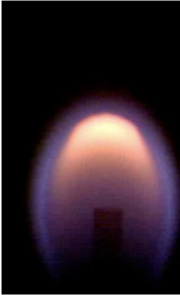
Figure 8. Image of a gas-jet diffusion flame (in air at ambient pressure) from a test conducted in NASA's 2.2 Second Drop Tower. The flame is being forced downward by the electric field between the burner and an electrode mesh, which is at +2 kilovolts and is down-stream of the burner.
