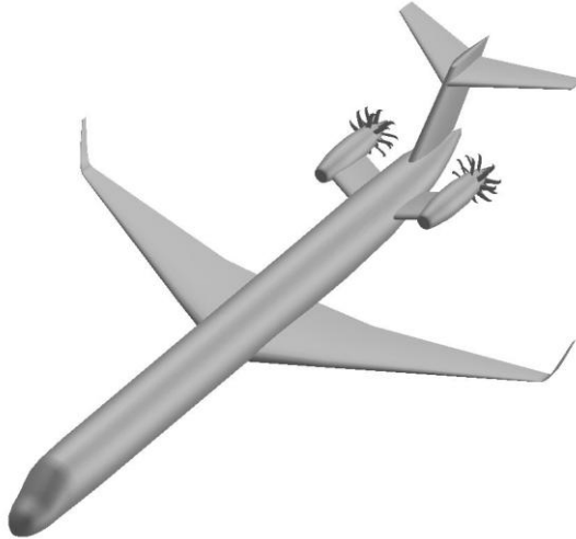
Figure 4. Basic Advanced Single-Aisle Transport configuration with rear-mounted open rotor engines (ASAT-or).
