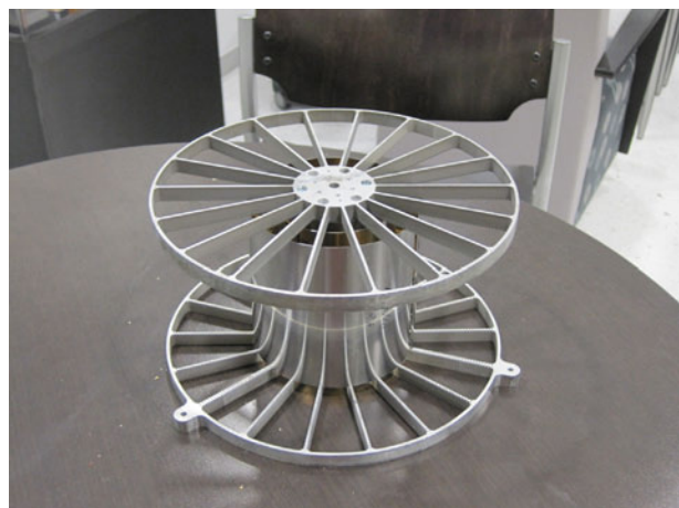
First integration test of the XACT optics with the spider assembly.
