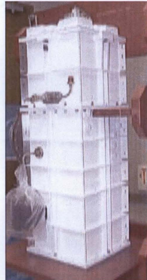
Completed ASRG Engineering Unit
