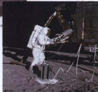
Alan Bean removing SNAP-27 fuel container from LEM
