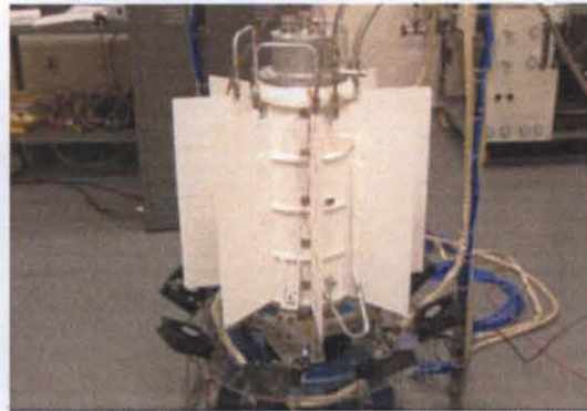
Figure 26. Multi-Mission RTG (MMRTG). Cutaway schematic of power unit on left. MMRTG Qualification Unit undergoing tests on right.
