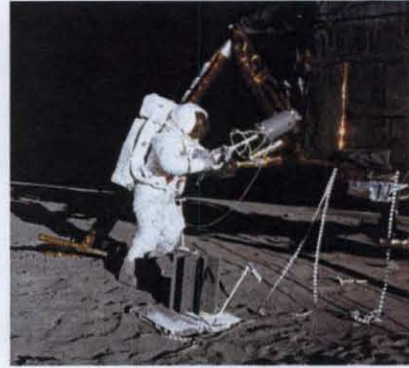
Figure 15. Use of SNAP-27 on the Moon. Alan Bean deploying SNAP-27 on Apollo 12.
