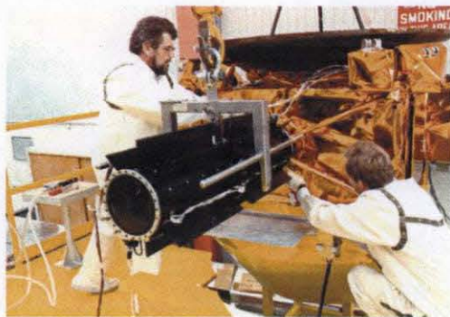
Figure 23. Ulysses spacecraft. Installation and checkout of RTG on left. Artist concept of vehicle on right.
