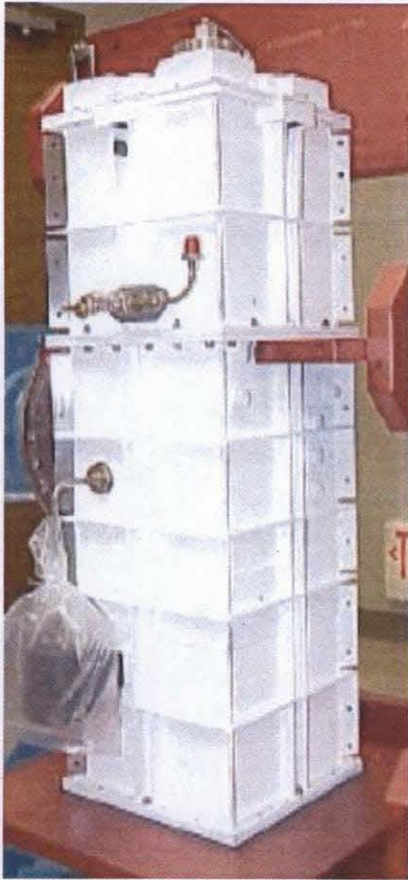
Figure 30. ASRG Engineering Unit.
