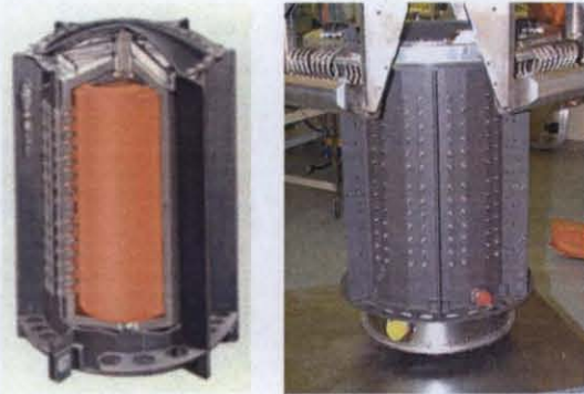
Figure 16. MHW-RTG. Cutaway view on left. Installation in test fixture on right.
