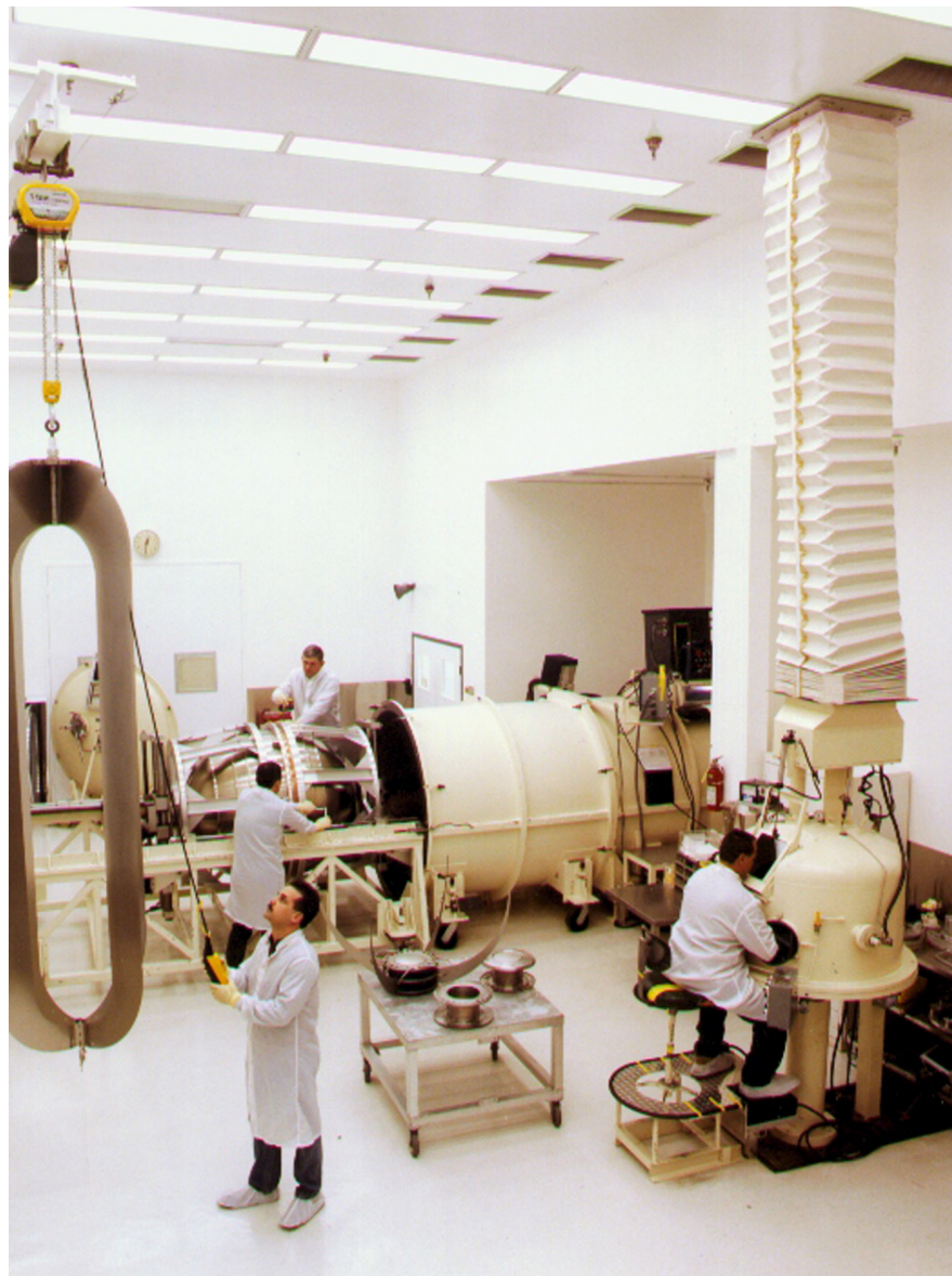
Employees work in the weld chamber for the assembly of the space shuttle auxiliary power unit (APU) hydrazine tank. The titanium hydrazine propellant tank is used on the space shuttle APU and is manufactured at ATK's Commerce, California, facility.
