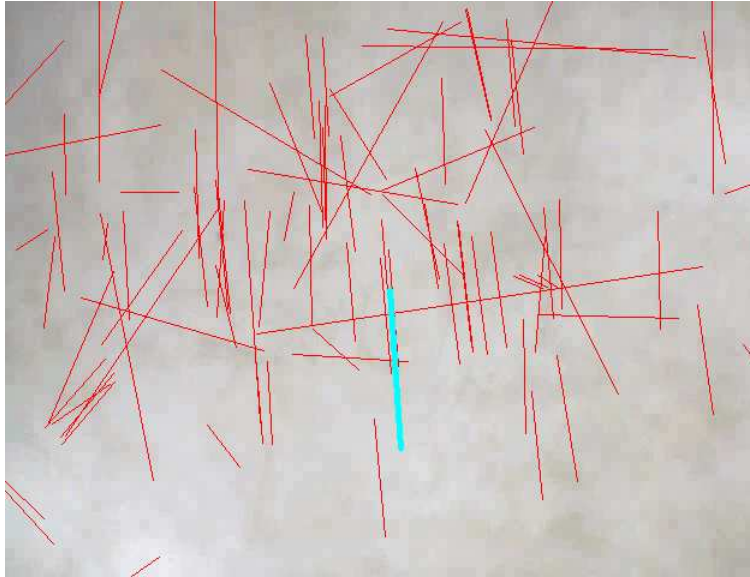
Figure 1. Optical flow results on a textured surface. The red lines depict offsets for tracked features. The bold cyan line in the middle indicates the estimated result of all the tracked features in the image.
