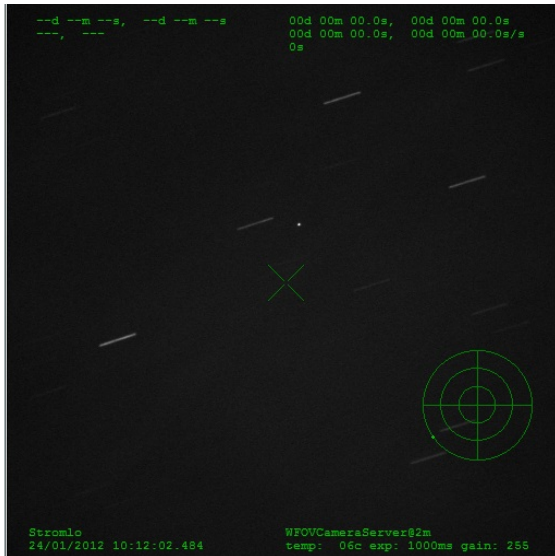
Fig. III: Picture of EOS Mt Stromlo Satellite Ranging System tracking object 21801 in front of the starfield.
