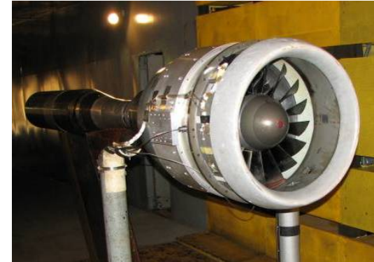
Microwave sensors installed on the NASA Turbofan Test Rig at the GRC's 9x15 LSWT
