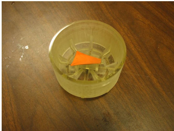
Figure 2.b. Stage 2 blade mounted in sabot.
