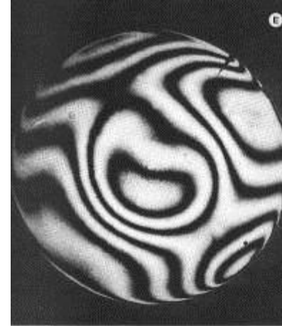
This Deformable Mirror - Before Active Optics System Activated
