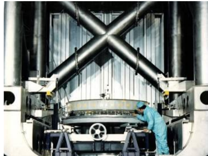
Start of Small Tool Computer Controlled Polishing (I saw this)
