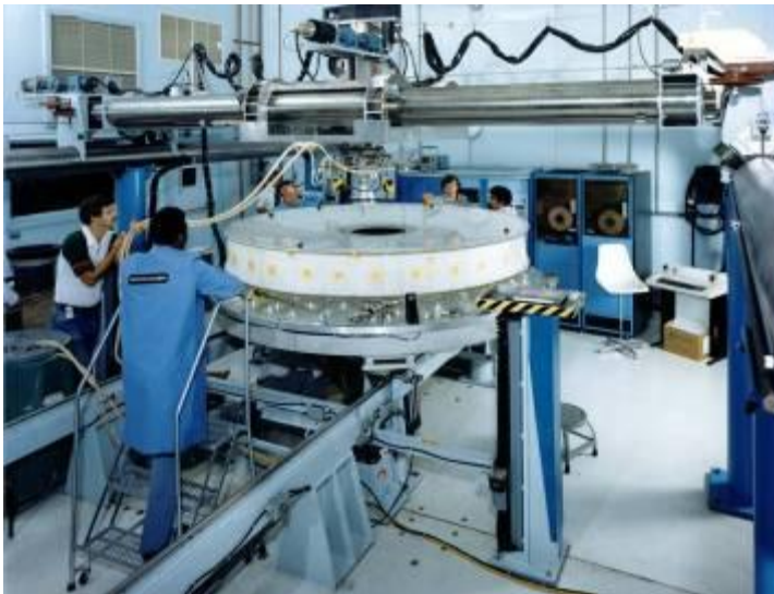
Start of Small Tool Computer Controlled Polishing (I saw this)
