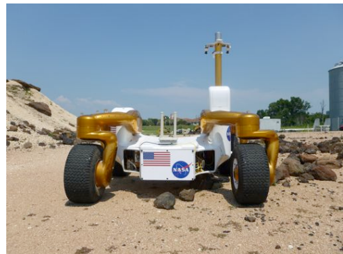
Figure 1: The Centaur2 rover at NASA JSC's Rockyard test site. Note the modular navigation mast installed on the right
