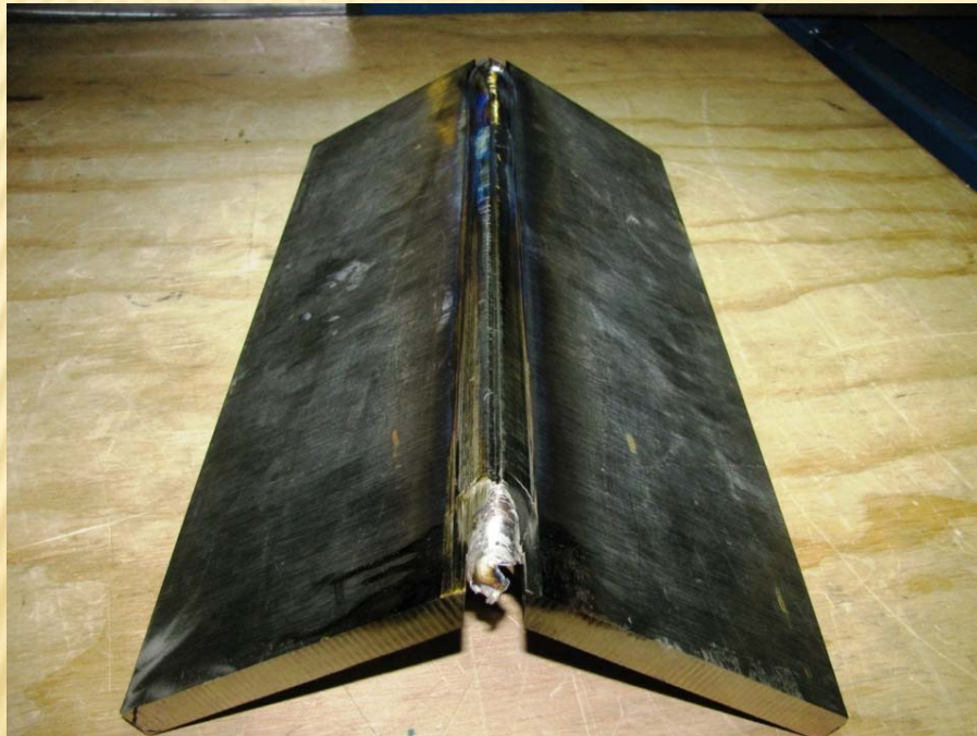
CP Ti .500-in thick angled weld - outside
