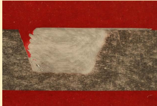
Sample 12-2 Bead on Plate
