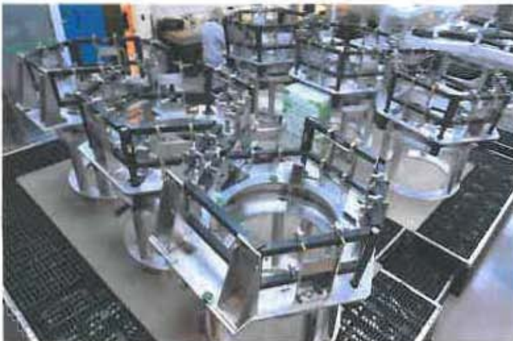
Wing Structures being built on Tooling
