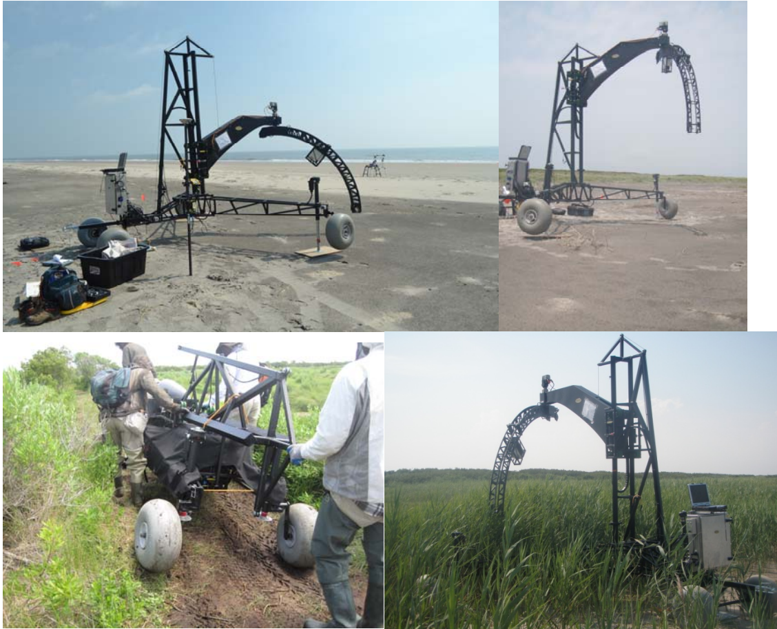
Figure 1. (Top, left) NRL GOPHER at the VCR'11 experiment during a measurement cycle; (top, right) the zenith arc can be adjusted to different heights to accommodate variable terrain or vegetation canopy heights (bottom, right). (Bottom, left) the GOPHER chassis converts to a compact form for transport across Hog Island during VCR'11.
