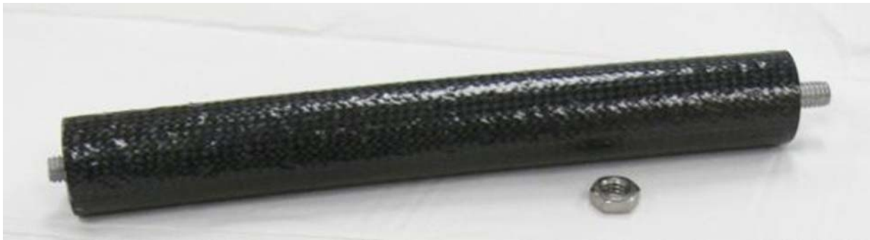
Figure 13: Composite strut for penetration testing.
