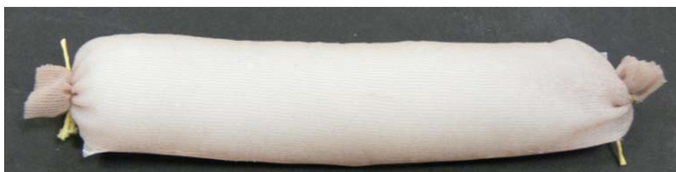
Figure 14: Aerogel bead package
