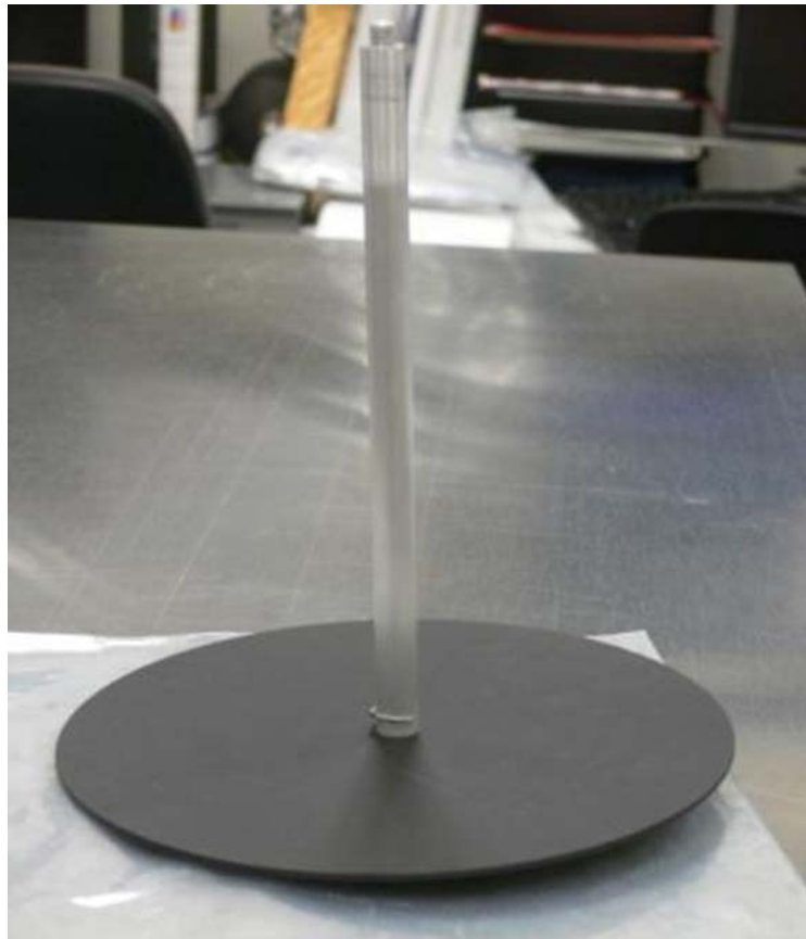
Figure 5: Passive heater attached to the half inch diameter strut
