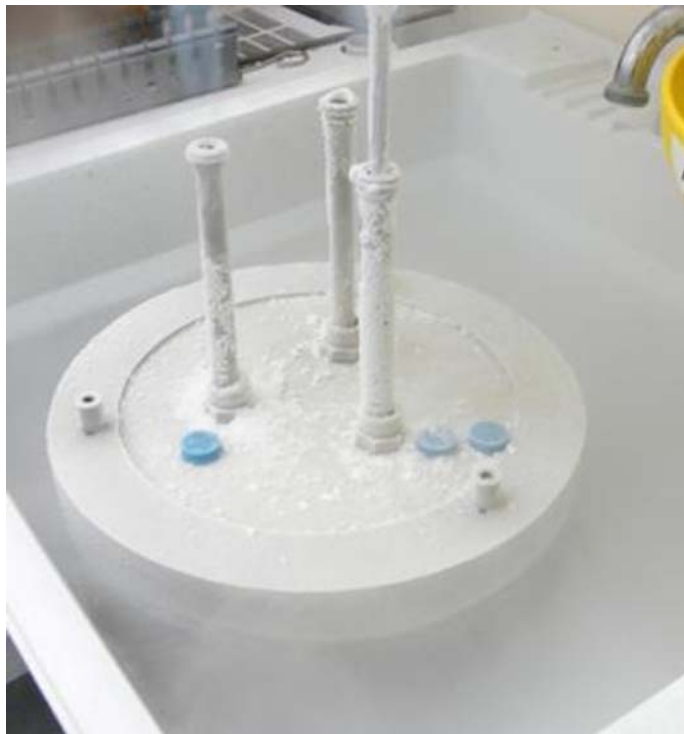
Figure 4: Cryostat-600 cold mass during liquid nitrogen cold shock
