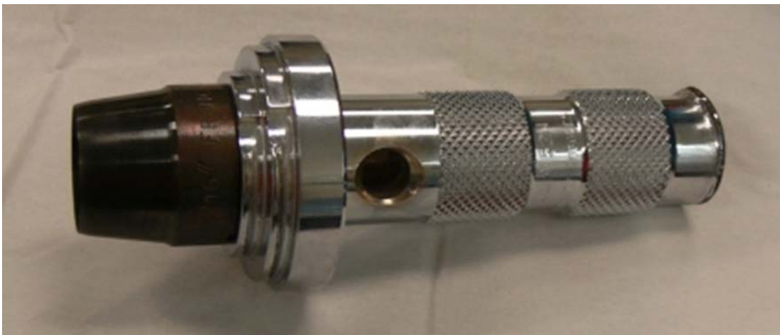
Figure 10: Punch used to insert holes into MLI blankets
