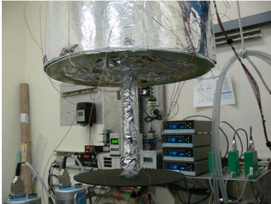
Figure 34: Composite strut installed on calorimeter with a Cryo-Lite buffer
