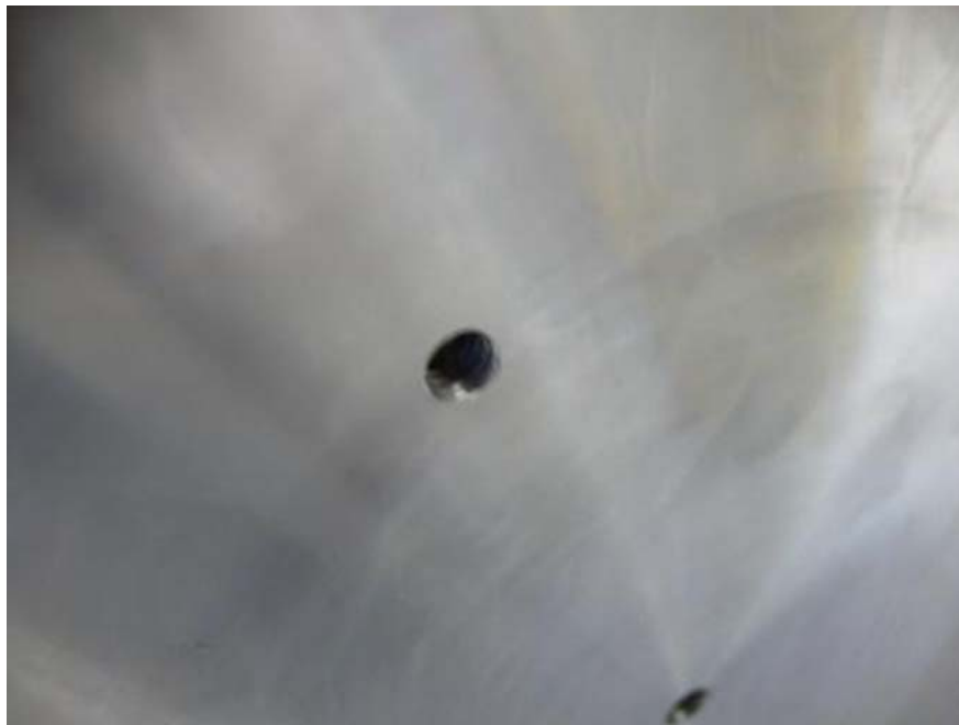
Figure 12: Threaded taps on the bottom of Crysotat-600
