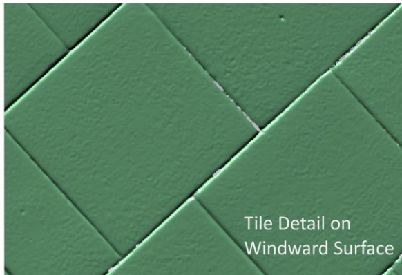
Figure 2. OML surface detail images depicting several tiles, and tile to tile step and gap region.
