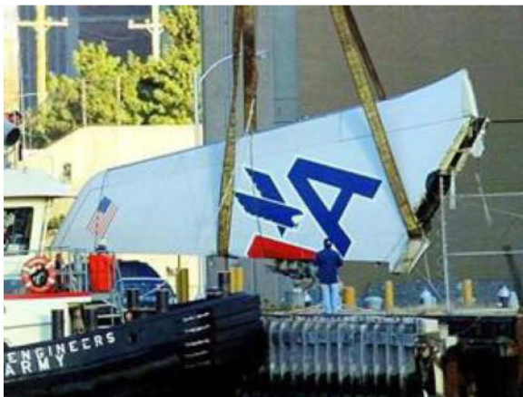
2001, AA587 Airbus A300 vertical stabilizer and rudder separated in flight due to excessive rudder input in response to wake turbulence
