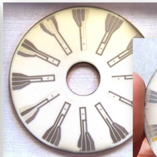
Early trials included Type-R thermocouples
