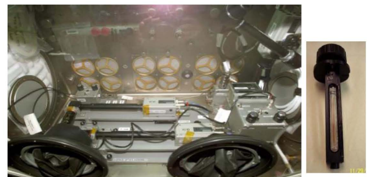
InSPACE in MSG with Vial Assembly containing MR fluid on right
