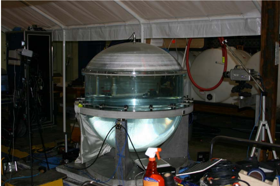
Figure 8: Ares I US LOX Tank Model in Test Bed.
