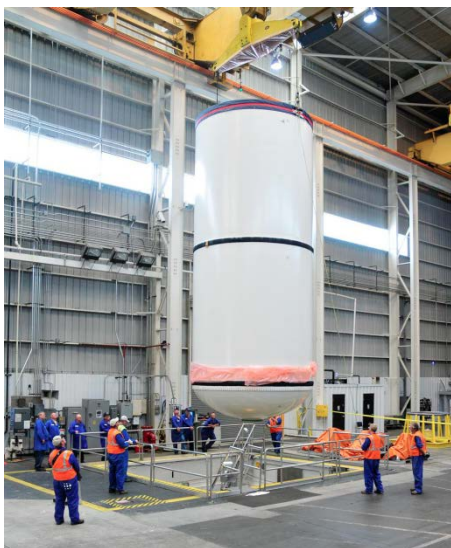
Fig. VIII. Booster qualification motor casting.
