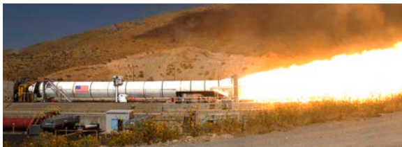
Fig. VII: A 5-segment booster development test.
