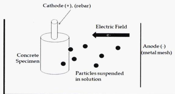
Fig.2 Graphical representation of electrophoresis
