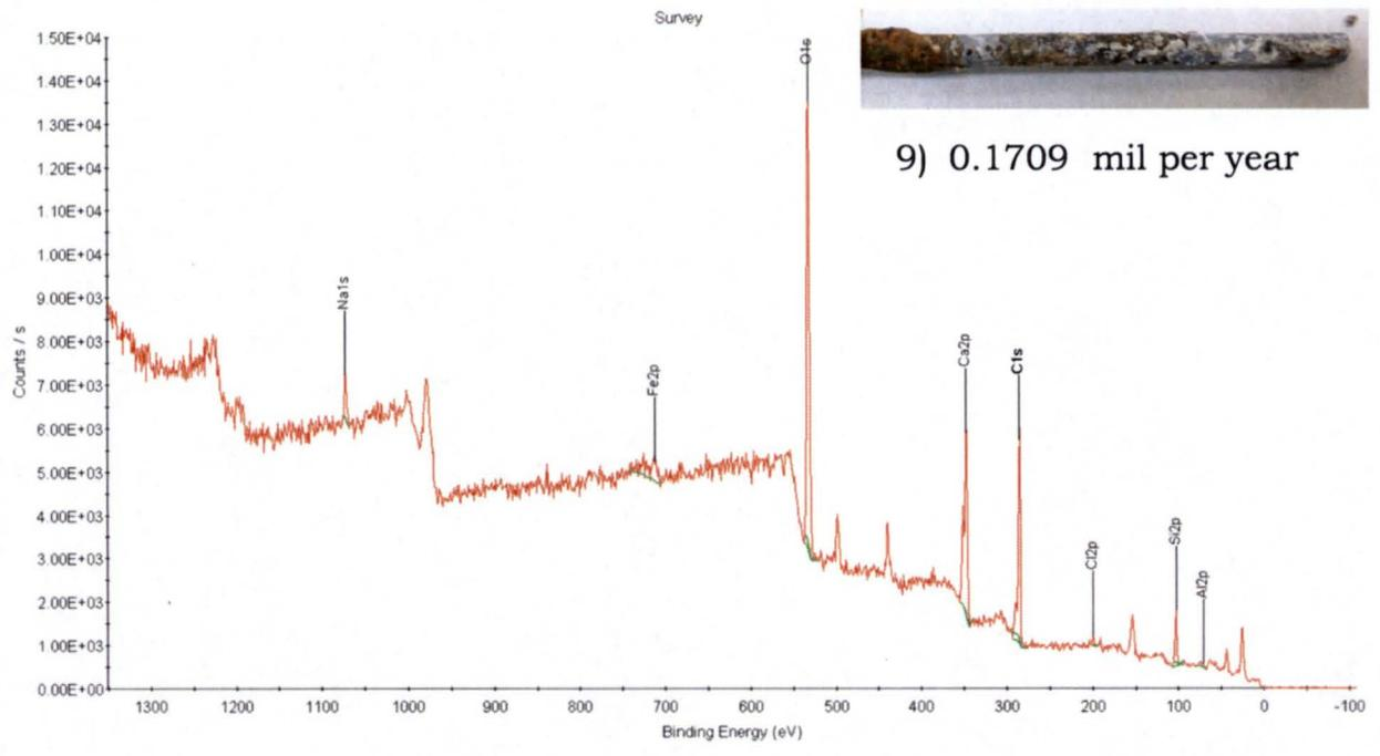
Fig.14 XPS of beach specimen 9 (atmospheric exposure)
