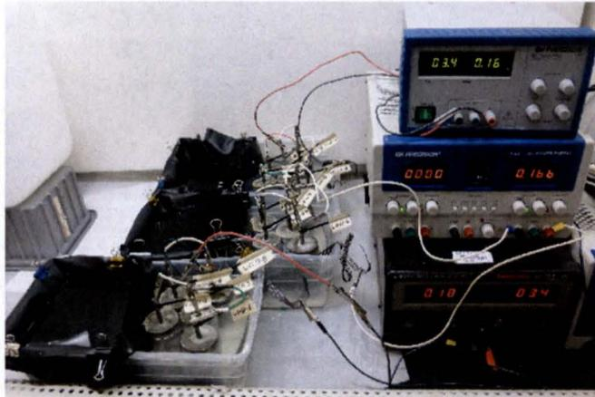
Fig.3 Specimens submerged in solution, and exposed to an electrical current.
