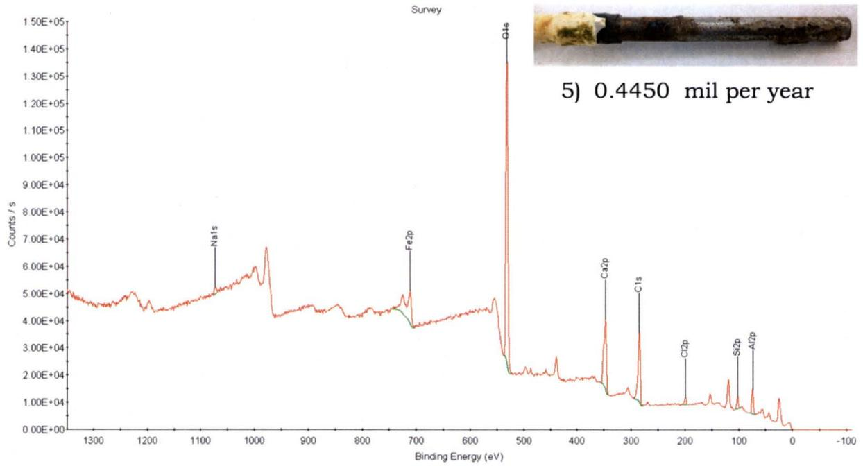
Fig.10 XPS of beach specimen 5 (atmospheric exposure)
