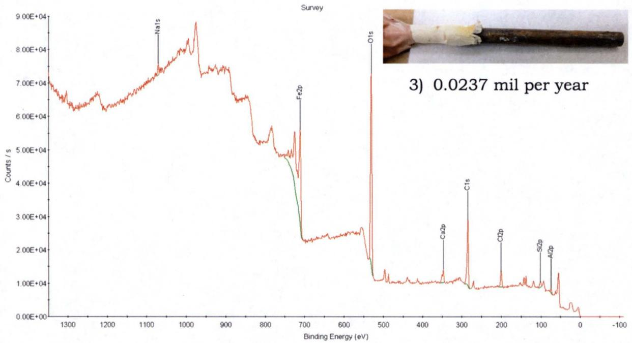
Fig.8 XPS of beach specimen 3 (immersed in seawater)
