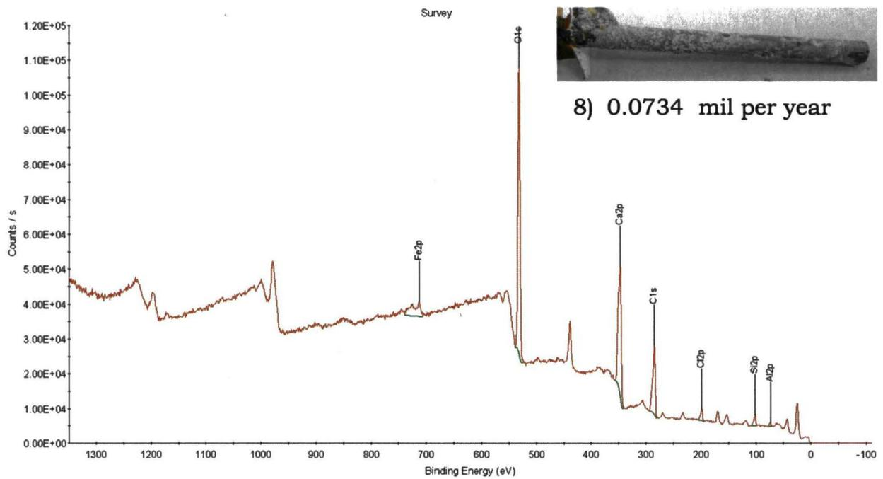
Fig.13 XPS of beach specimen 8 (atmospheric exposure)
