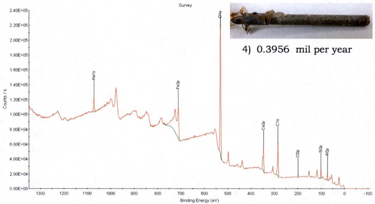
Fig.9 XPS of beach specimen 4 (atmospheric exposure)
