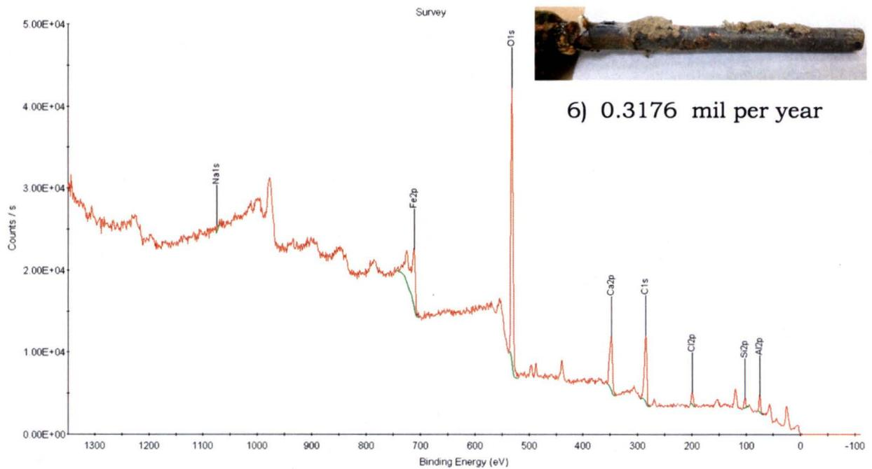
Fig.11 XPS of beach specimen 6 (atmospheric exposure)
