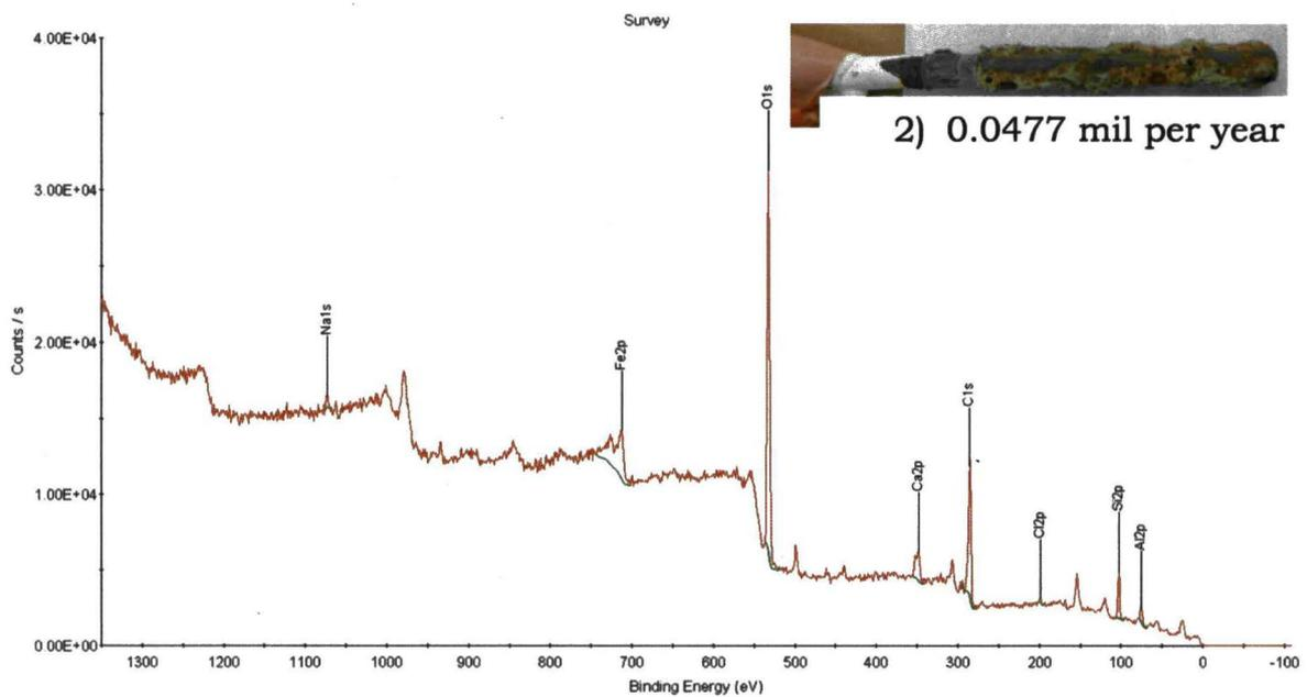
Fig.7 XPS of beach specimen 2 (immersed in seawater)
