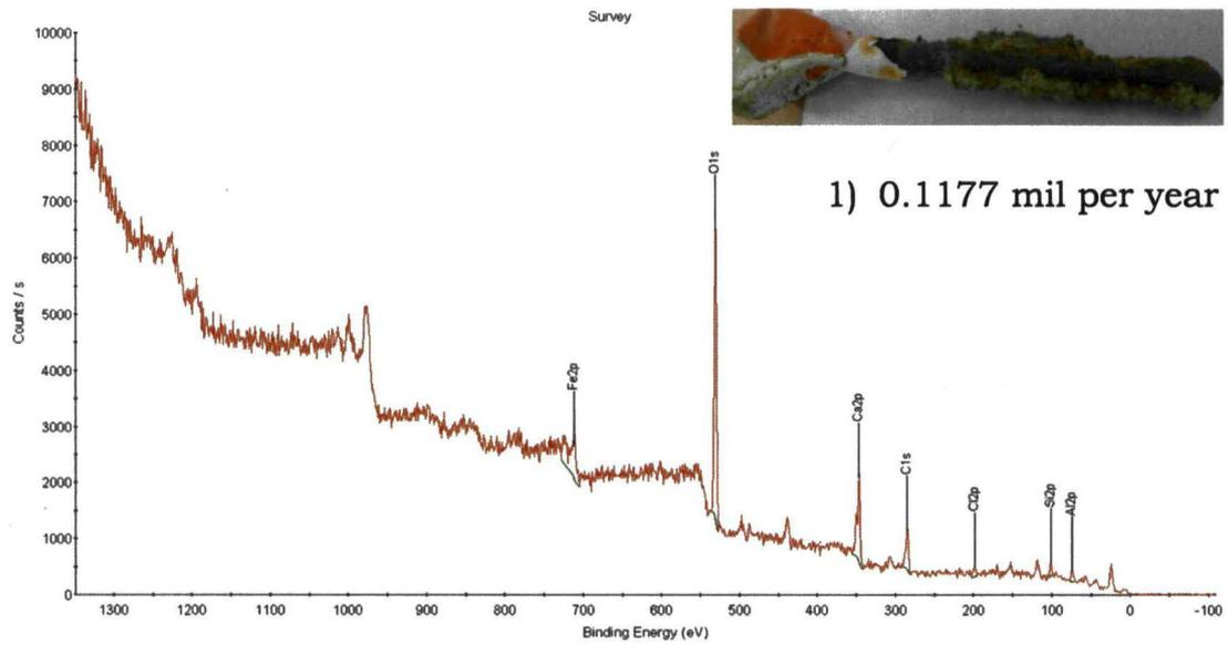
Fig.6 XPS of beach specimen 1 (immersed in seawater)
