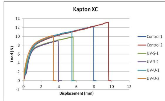
Figure 4. Load versus displacement curve for Kapton XC
