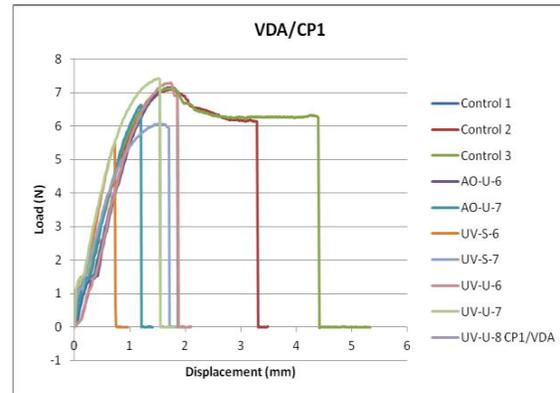
Figure 7. Load versus displacement curve for CP1/VDA
