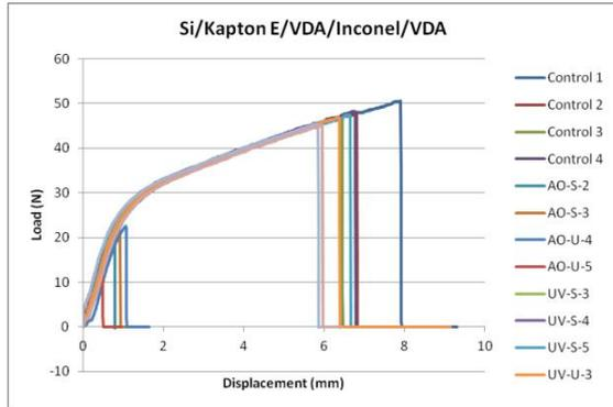
Figure 3. Load versus displacement curve for Si/Kapton E/VDA/Inconel/VDA
