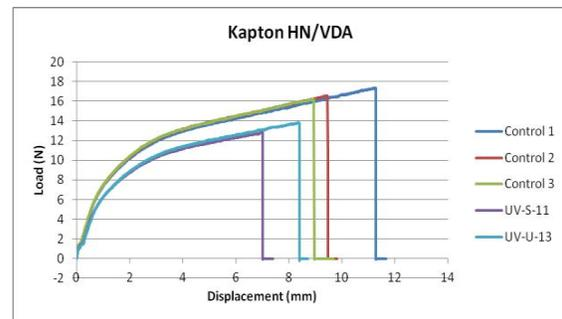
Figure 5. Load versus displacement curve for Kapton HN/VDA
