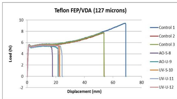
Figure 2. Load versus displacement curve for 127 micron thick FEP/VDA
