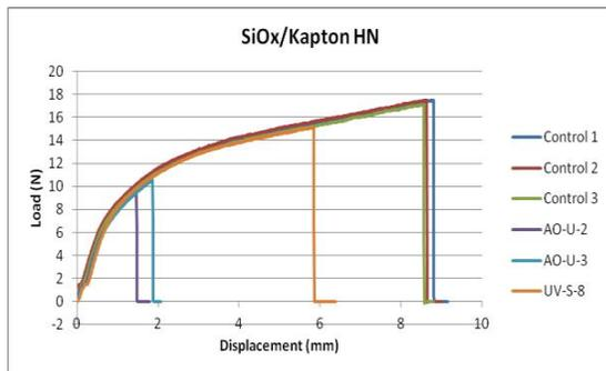
Figure 6. Load versus displacement curve for SiO<sub>x</sub>/Kapton HN.
