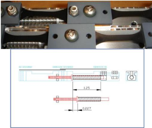
Figure 1. Photo of stressed (left) and unstressed (right) sample holders from above, and a side view drawing of a holder showing the unstressed sample position on the left and the stressed on the right. (Dimensions are in inches.) The stressed sample is fixed on the left side and allowed to move to the right by having the mount hole on the right slotted. Tension is supplied by compression of the spring.
