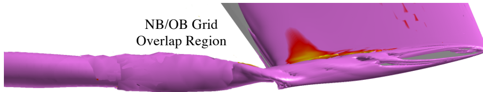
Figure 24 Tip vortex formation for the AMR2 wake grid. TRAM rotor in hover: M_{tip}=0.625 , \theta=14^\circ , and Re=2.1 million.
