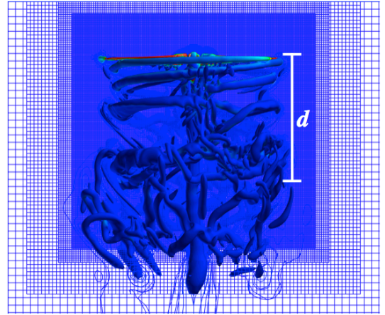
b) Turbulent rotor wake.
