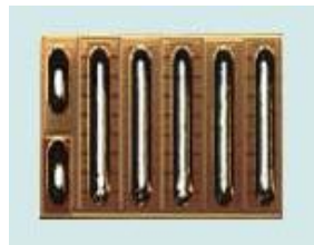
Figure 1. EPC transistor structure with solder bumps
