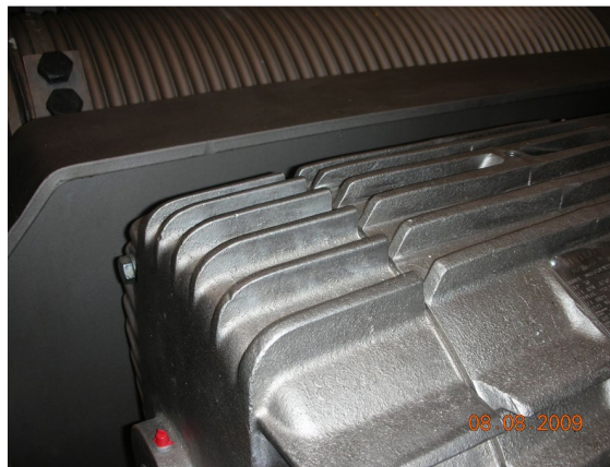
Figure 9.—Main hoist motor casing after electroless Ni-plating.
