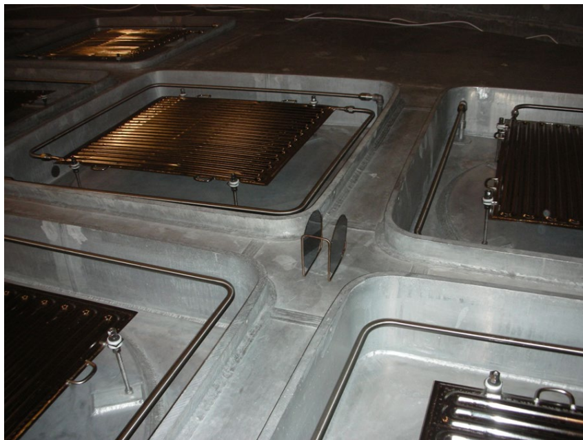
Figure 11.—Silicon wafers mounted among scavenger plate wells.
