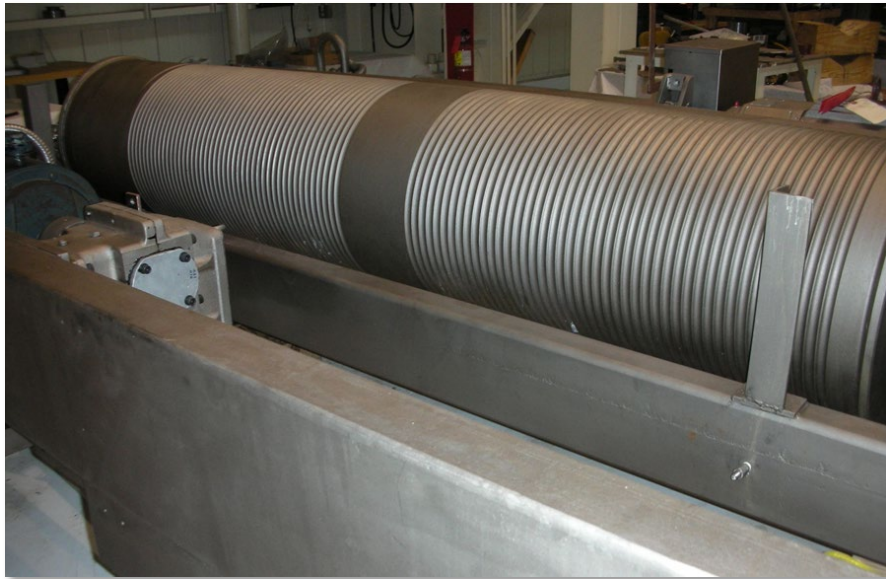
Figure 8.—Main hoist drum and trolley after electroless Ni-plating.
