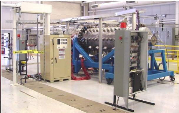
Non-Nuclear Hot-Hydrogen Component Tester using Induction Heating to Simulate Fission (NTREES)
