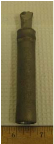
Piece parts of integrally cladded HIP sample (top). Cladded HIP sample post HIP
