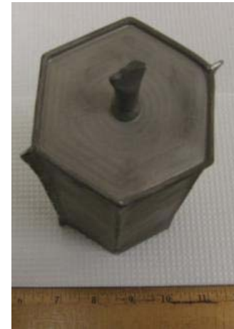
Molybdenum mandrel assembly for 331 Hexagonal demonstration
