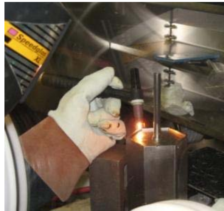
Top end cap welding of 331 Hex demo
