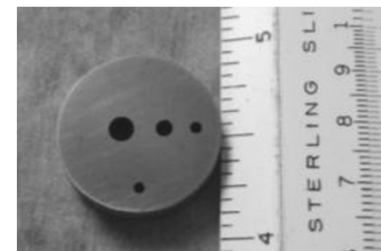
EDM Trials on W- \text{CeO}_2 Specimen
