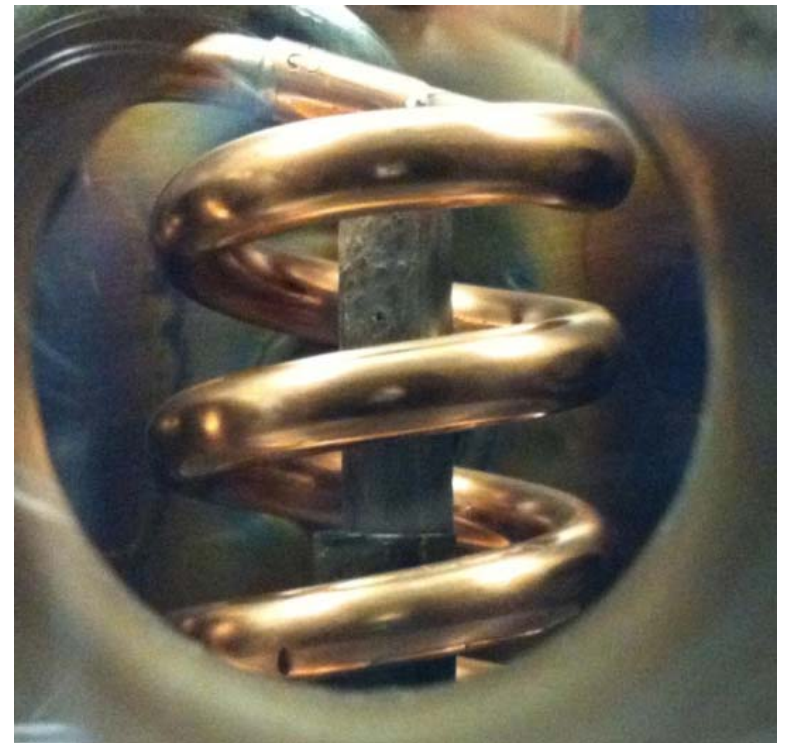
W/Re sample loaded into heating coil as viewed through the pyrometer viewport
