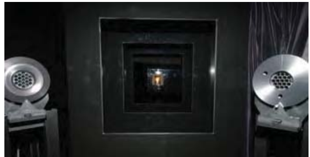
Fig. 53. A view from the plaque of the radiance bench toward the calibration standard (dimly lit for clarity). The OXL prototype is on the left side and an EML sensor is on the right side with the spectrograph aperture oriented downward (6 o'clock position). Both instruments are positioned with kinematic mounts. All reflections are caused by the camera flash.
