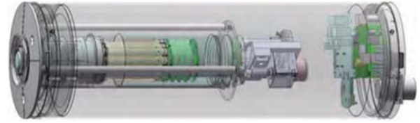
Fig. 52. A simplified technical drawing of an EME (or OXE) following the approach in Fig. 51. The primary new component is the plano-convex lens (white) immediately left of the microradiometers (brown) and the cosine collector on the aperture end plate (blue).
