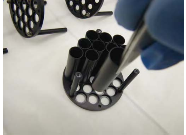
Fig. 17. The initial assembly of the first of four layers of Gershun tubes, made from hollow black cylinders, which are stacked to control the FVA.
