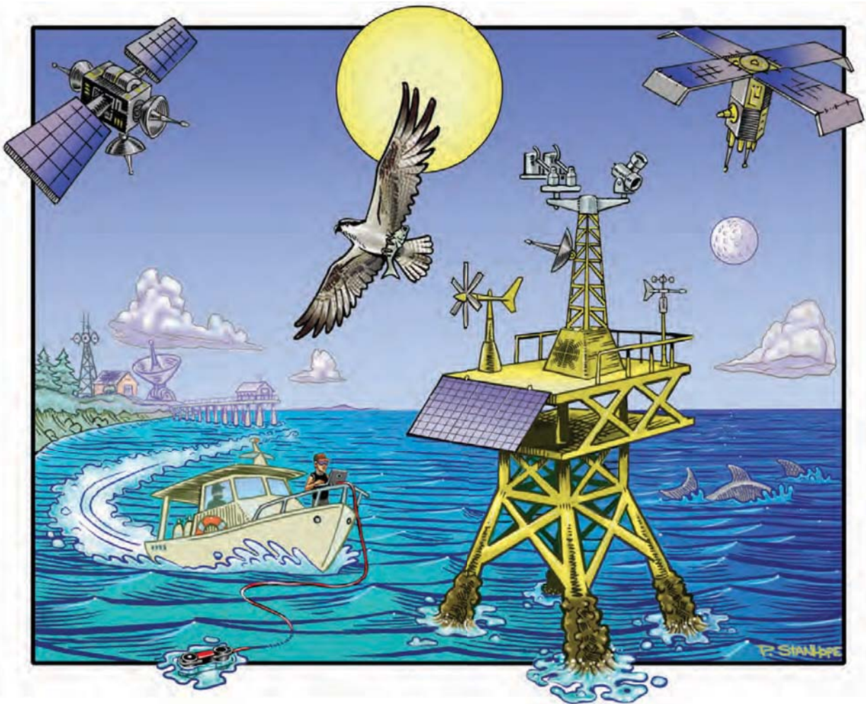
Fig. 2. Deployment of the OSPREy system with many of the components required for operations: two EMR dyads at the top of an offshore tower measuring the atmosphere and the ocean; an ocean color satellite (SeaWiFS) sampling the on- to off-shore gradient (green to blue) in productivity; the Sun and Moon as calibration targets for SeaWiFS and OSPREy; a telecommunications satellite for data telemetry from the platform sensor suite (including meteorological sensors), which are all powered by solar panels and a wind generator; a shore-based calibration and logistical support facility, including test capabilities at a pier; and monthly validation (including in-water AOP profiles) and maintenance visits with a small boat.
