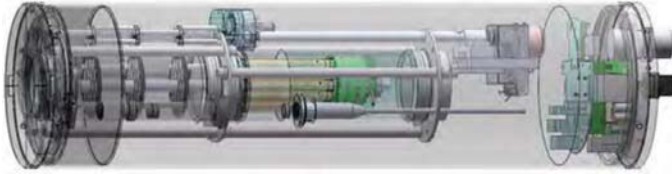
Fig. 51. A simplified technical drawing of an EML radiometer. The core of the design is the cluster of microradiometers (brown) left of the aggregator stack (green) with filter-wheel assembly above, fiber and spectrograph (pink) to the right, and camera below. The electronics positioned near the end cap primarily support the spectrograph. Some details are omitted (e.g., wiring and insulation) for clarity.
