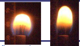
N 2 flow makes candle flame longer, it does not put it out.
