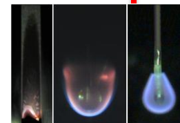
Flat, Spherical, and Cylindrical samples (L to R) burning in 1-g
