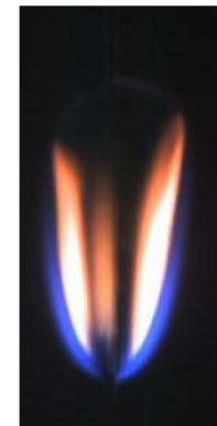
Side view of a low-g flame on a thin paper sample in a concurrent convective flow
