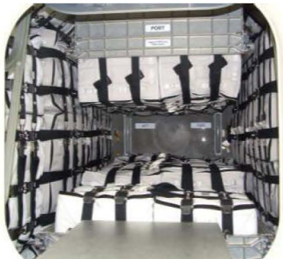
Load experiment into Cygnus PCM
