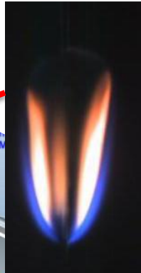
Side view of a low-g flame on a thin paper sample in a convective flow
