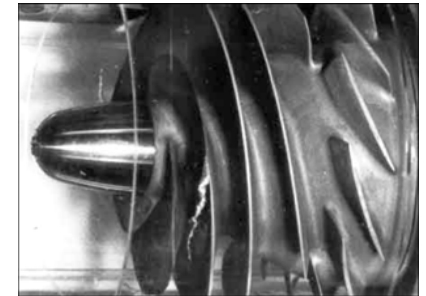
Pump Waterflow Test Article
