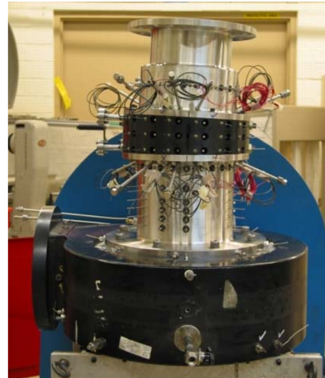
Low pressure pump with upstream main propulsion system element simulation
