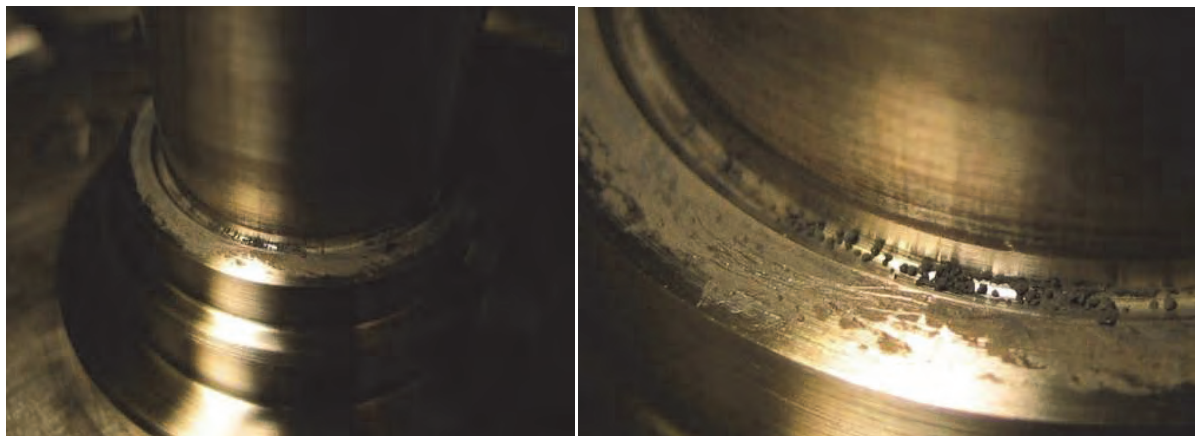
Figure 6. Similar fretting wear found in FWA qualification unit bearing shaft. The 0.127-mm (0.005-inch) nodules collected from the bearing relief consisted of nanometer-sized particles of titanium from the shaft and iron from the bearing and had the consistency of dry powder that smeared when touched.
