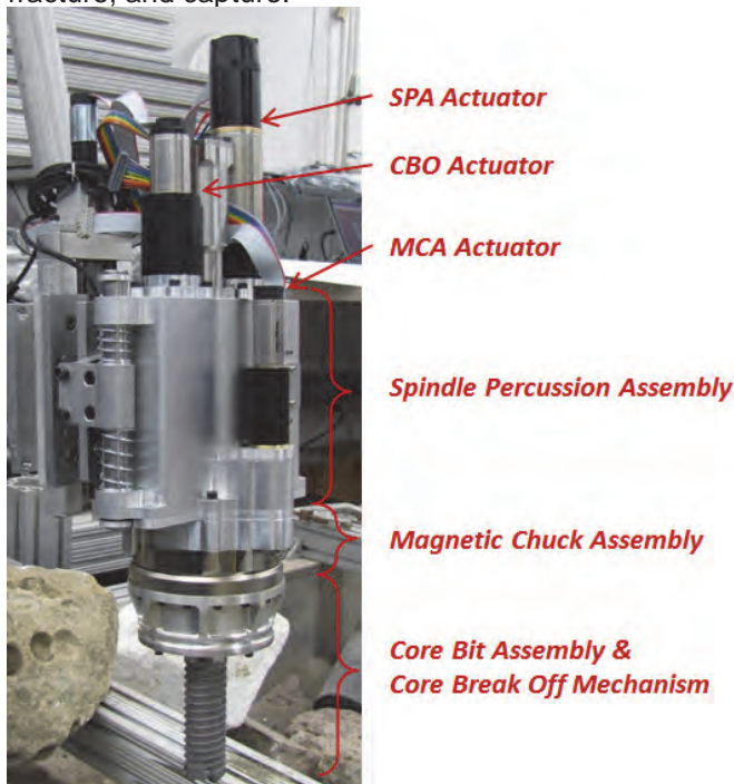
Figure 5. Rotary Percussive Sample Acquisition Tool (SAT)
