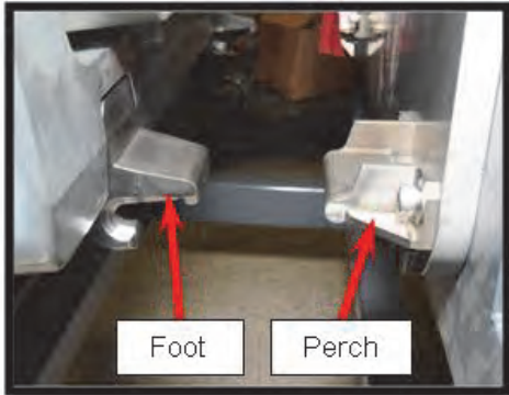
Pivot Feet Prior to Connection
