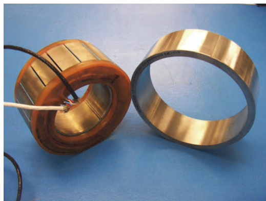
Figure 13. Photo of the G Motor - Rotor is encapsulated in titanium ring
