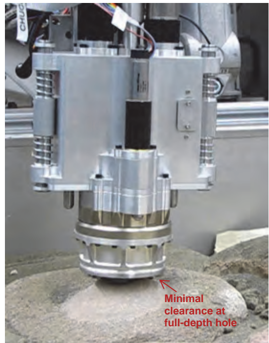
Figure 15. Tool cannot accommodate large surface irregularities or drilling at off-normal angles due to minimal clearance between bit housing and rock.
