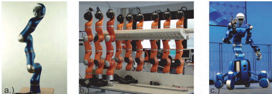
Figure 5: a.) LWR III, b.) LWR as a KUKA product, c.) modular robot system "Justin" with 54 DOF
