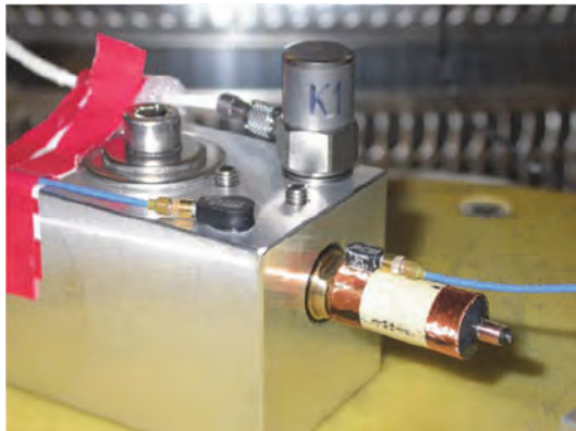
Figure 4: Test setup for the random vibration test conducted on the RE13 winding
