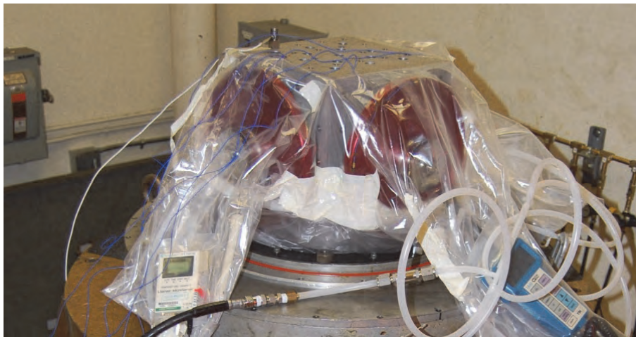
Figure 16. Second vibration test of the TiN-coated, WCC-coated, and bare (control) titanium shaft configurations. Note the dry air input as well as the humidity meters for each configuration.
