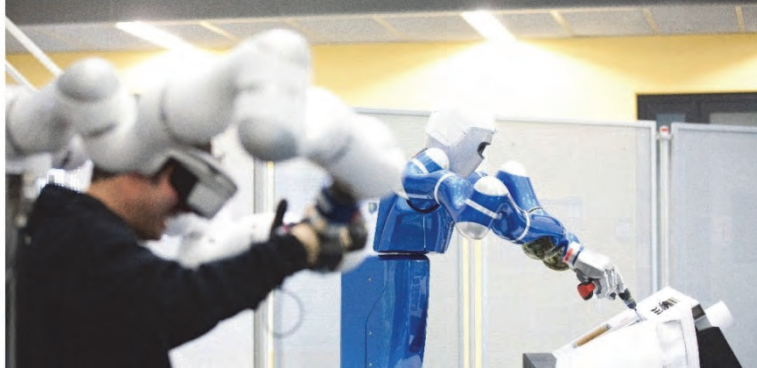
Figure 1: Teleoperator using a head-mounted display to get 3D visualization and lightweight Robots (LWRs) as haptic input device with force feedback and "Justin" in telerobotic operation
