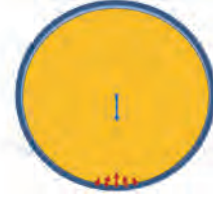
Figure 11b. Start of tipping, normal force on bottom is a small contact patch ( F_b = 0 )
