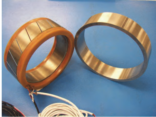
Figure 18. Photograph of the H motor with the lamination skew
