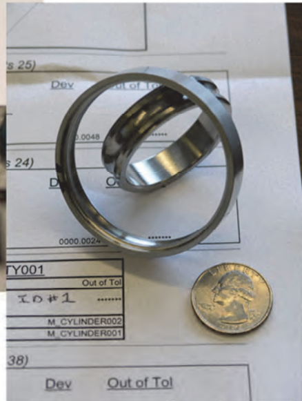
Figure 8. Plunge turning of 60NiTi race rings using a carbide tool profiled to match the desired race geometry using wire EDM.
