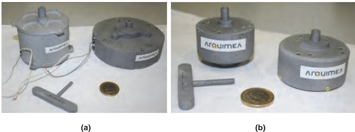
Figure 12. Built demonstrator of the both Arquimea Pin Puller versions: (a) devices of 500 N of stroke force; (b) devices of 100 N of stroke force.
