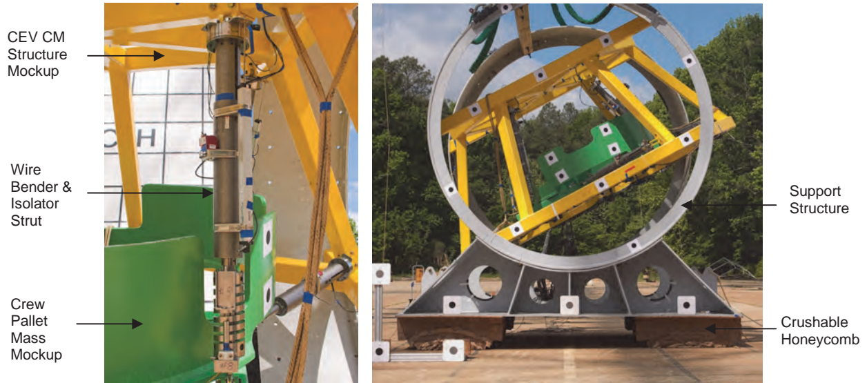
Figure 7. Attenuation Strut in Assembly (Left); Drop-Test Fixture (Right)
