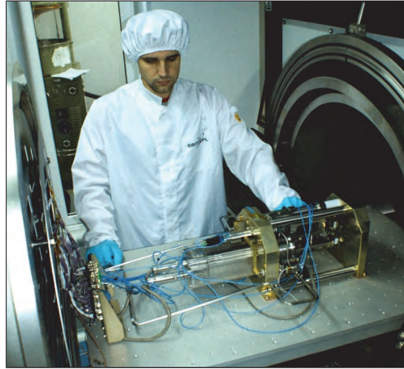
Figure 10. Pin-on-Disk tribometer mounted in the SRC thermal-vacuum chamber
