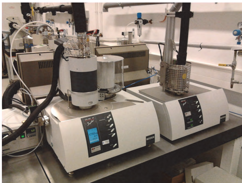
Figure 1. Furnace (left) and mass spectrometer (right).
