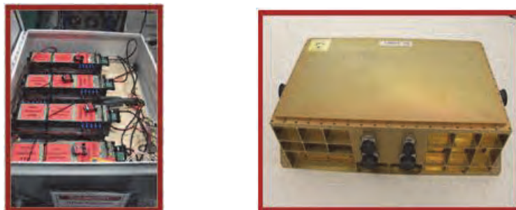
Figure 7. Developmental Lithium Ion Battery Supply (left) and Common Controller
