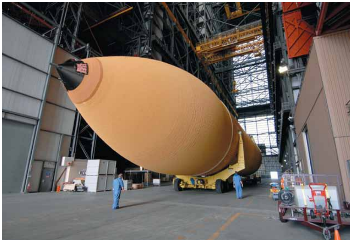
An external tank holding liquid hydrogen and liquid oxygen for the now-retired space shuttle arrives at the Vehicle Assembly Building at Kennedy Space Center. To ensure safety, NASA studied and tested the materials used on the tank for ignitability and flammability.
