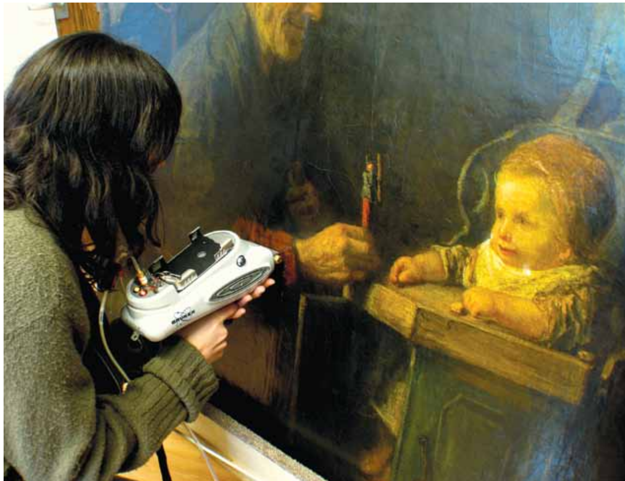
Bruker AXS’s XRF scanners quickly and easily identify the elements of an object down to parts-per-million—sufficient to analyze NASA spacecraft components or authenticate works of art.
