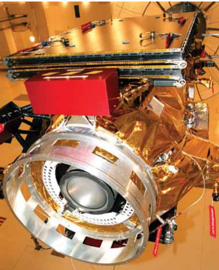
Deep Space 1 was a spacecraft designed to test a dozen different space technologies, including a solar array that focused sunlight on a smaller solar cell to generate electric power.
