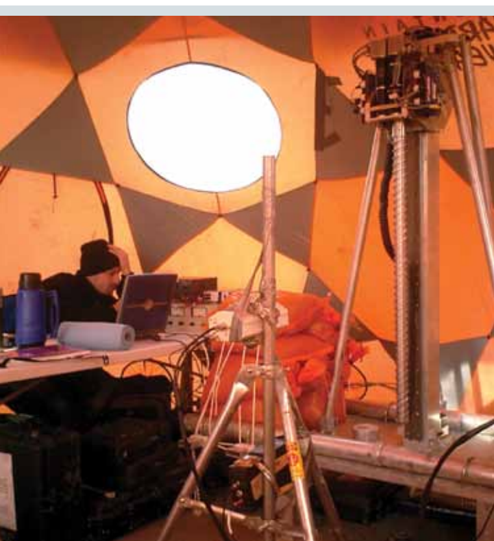
The DAME drill during summer field tests on Devon Island, NASA's Mars analog site. The devices at center are laser vibrometers that measure the movements and vibrations of the drill when in use.
