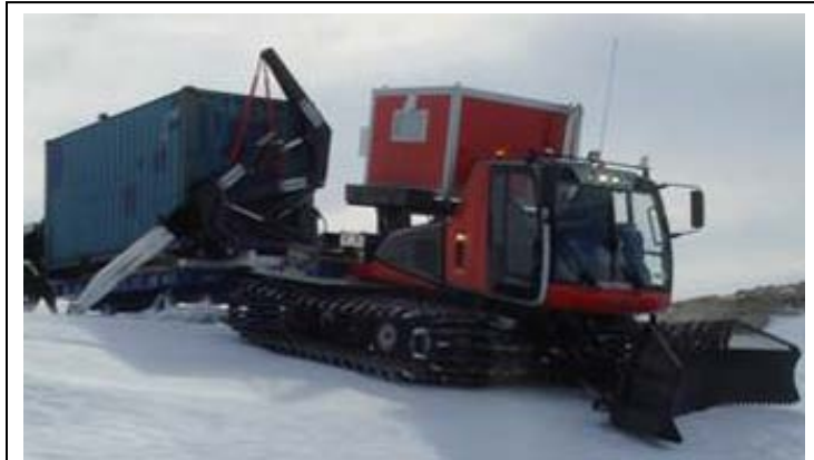
Prinoth Everest Power Antarctic preparing to transport a cargo container in support of the construction of the Princess Elisabeth Station. (Source: Johan Berte)
