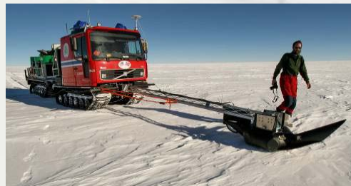
"The sniffer", a 400 MHz GPR
