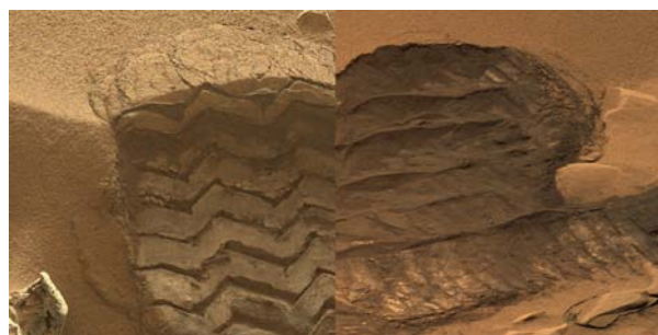
Figure 1: (a) left , Rocknest at Gale Crater, wheel imprint is ~40 cm wide, (b) right , Serpent at Gusev Crater, Spirit wheel width is 16 cm.
