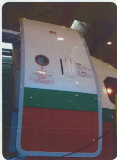
Service Door of Airbus 319 where Chrome-free Coatings were Applied
